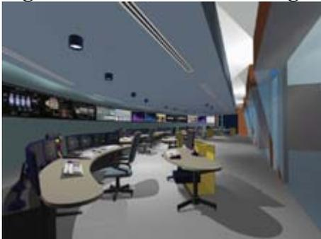
*Future control rooms, like the one shown here by Galen Crazz, Dept. of Architecture, University of Calif., follow ISO 11064 design guidance on workstation groupings, spacing requirements and visual display locations.*
